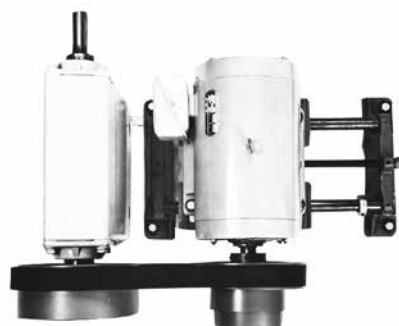
Adjustable Center V-Flat Drive Maximum Speed Position
