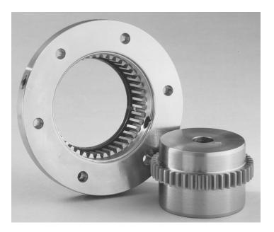
can approach 78 inches in diameter). AGMA specifies that flange gear couplings from size 1 to size 9 will match up half for half with other flange type gear couplings made to the AGMA standard dimensions. However, while the dimensional standard ensures compatibility of the face to face match between sleeve flanges, it does not assure matching torque or bore capacity.
