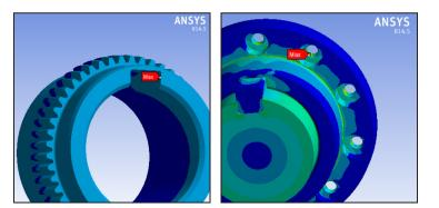
a battery of worst case conditions. High cycle coupling fatigue, high misalignment tooth fatigue, ultimate torque capacity, high torque reverse loading and seal contaminated environment life performance are just a sampling of the extensive validation testing performed. Comparing the results achieved during the physical testing to the predicted analytical performance confirmed the validity of the analytical models.
