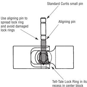
Joints 3/4" and smaller outside diameter have small pins riveted at the factory.
