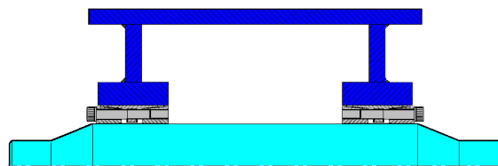
Conveyor pulley with Shaft Locking Device
