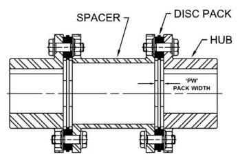
7.4 Carefully move the spacer into position between the hubs without allowing the spacer to impact against either hub. <u>Always</u> maintain support for the spacer until all bolts are in place.
