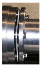
**7.15 Check the angular misalignment** by measuring the gap between the guard ring and spacer flange at four or more locations around the coupling, preferably at the 3:00, 6:00, 9:00, and 12:00 positions and compare these values with the 'PW'/Low value and the 'PW'/High value in Table-4. If any of the measurements fall outside this high/low range, make adjustments in the equipment alignment before continuing.
