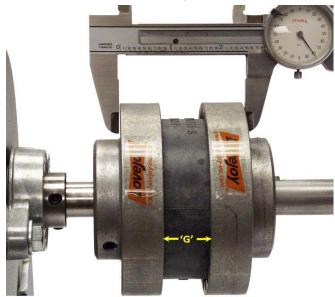
**6.11 Next, lay a straight edge across the top of the flanges** and note the space between the straight edge and the second flange. This parallel misalignment should be less than the 'Parallel' value listed in Table-4. If it exceeds this amount, realign the equipment to correct this condition. This will also work for angular misalignment.
