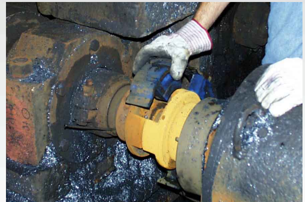
Easy to install the Urethane element
