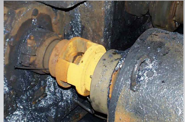
Jaws line up so the element is in shear
