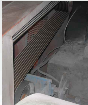
Multi-Groove V-Belt running on the Lovejoy ROSTA Heavy Duty Tensioner
