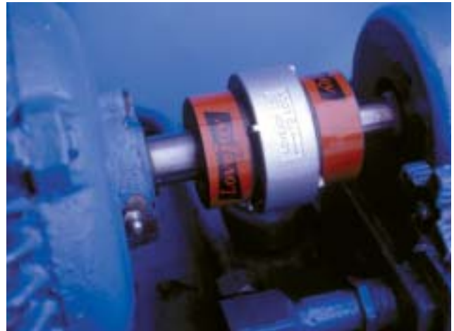
Step 4 Twist locking ring to secure.
