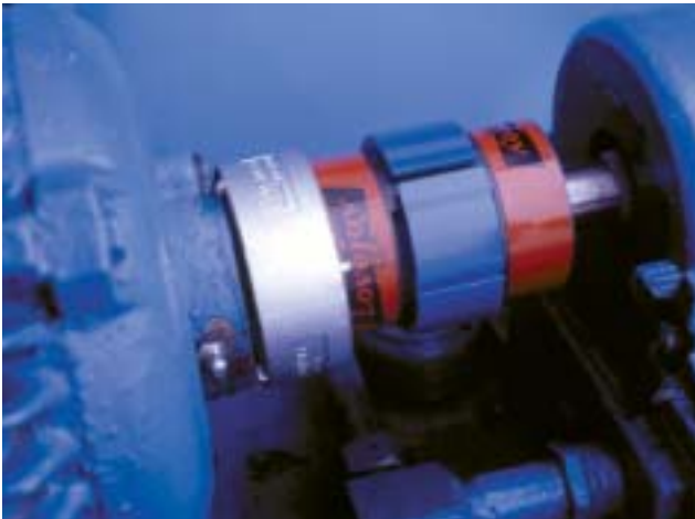
Step 3 Slide locking ring over element.
