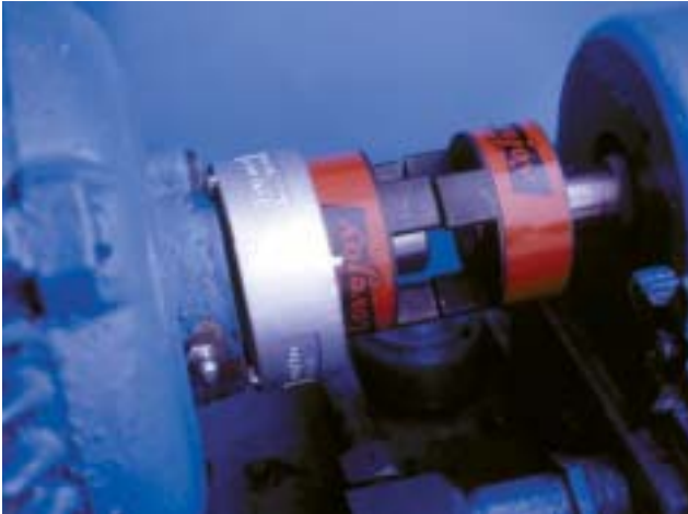
Step 1 Remove element and align hubs.
