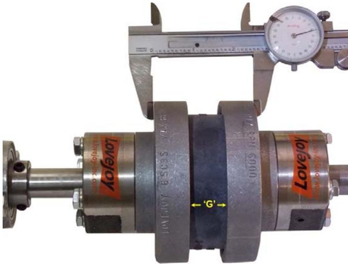
**6.11 Lay a straight edge across the top of the flanges** and note the space between the straight edge and the second flange. This parallel misalignment should be less than the 'Parallel' value listed in Table-4. If it exceeds this amount, realign the equipment to correct this condition. This will also work for angular misalignment.
